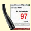
using HC-sniffer with cable and flexible detector head
