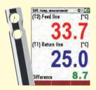
using thermocouples with 2 standard K-type sockets
