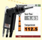
built-in electronic controlled heated probe shaft with soot filter
