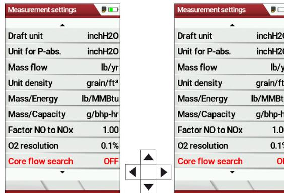
You can preselect whether a core flow search is to be carried out in the measuring programs before the start of the measurements.
