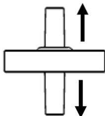
Observe the direction when installing the water stop filter
