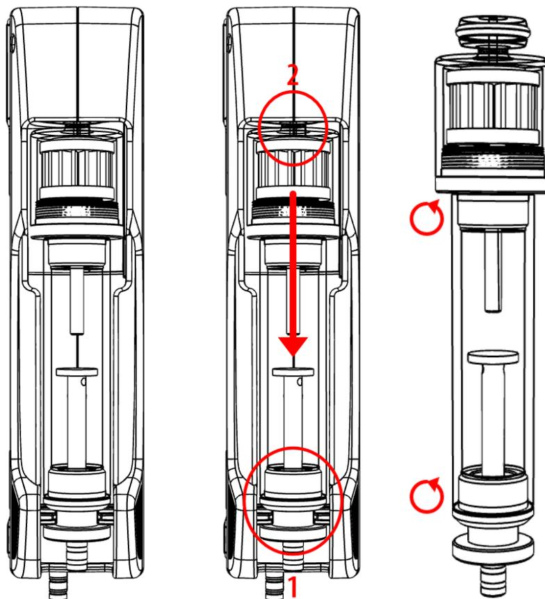
Remove the condensate separator by lifting it out from the groove (1) of the analyser. Then pull out the condensate separator downwards (2). Liquid discharged from the condensate separator may be slightly acidic.
