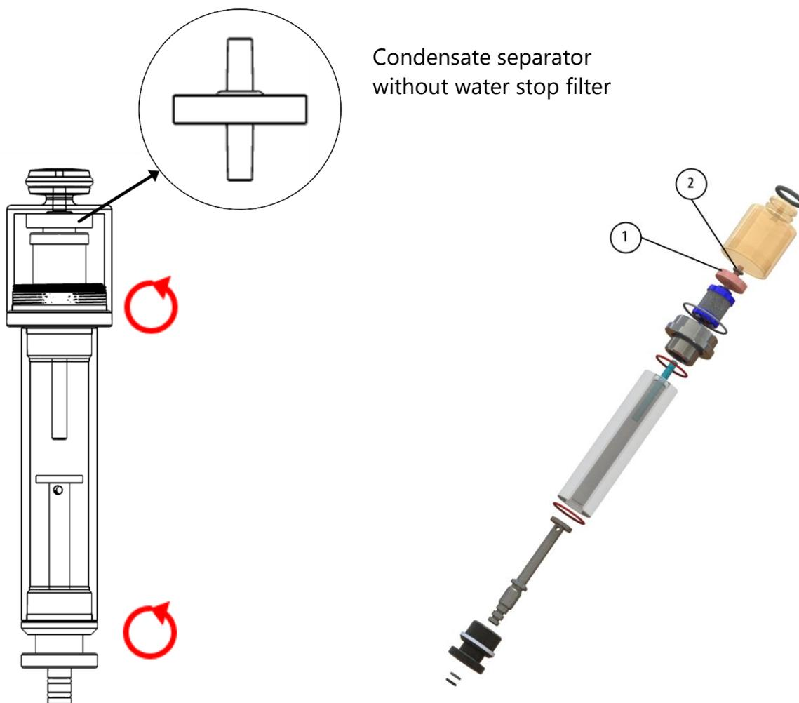
Condensate separator without water stop filter
