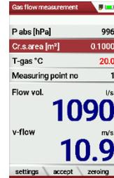
If you do not connect a temperature sensor, a value for T-gas of 20°C is automatically assumed.
