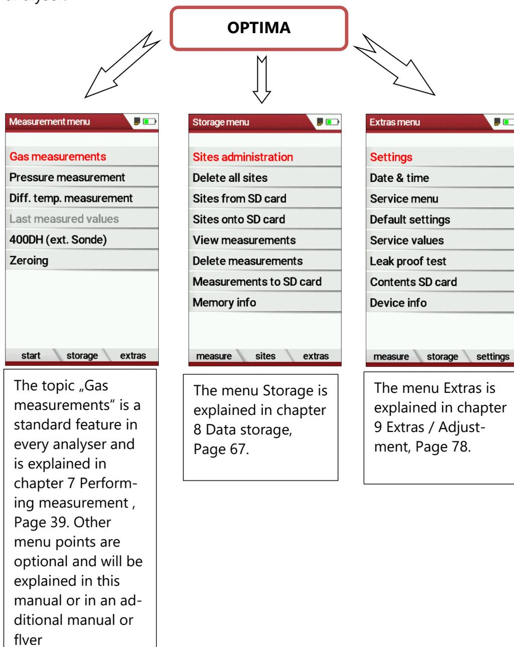
You can jump in between the 3 main menus with the 3 function keys (according to the displayed name on the screen).
