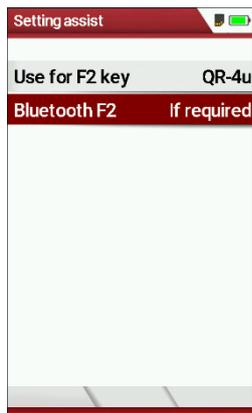
If you set Bluetooth to F2 "If required", measurement data will always be transmitted to MRU4u as soon as there is a connection between the analyser and MRU4u. The display in the measurement assistant changes automatically as soon as a connection is established between the analyser and MRU4u.
