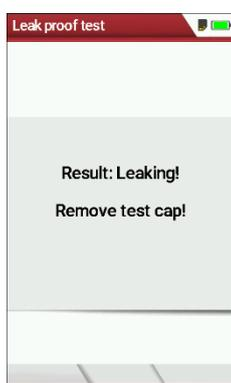
If the leak proof test is not passed, you must check the probe including the tubing and the condensate separator.
