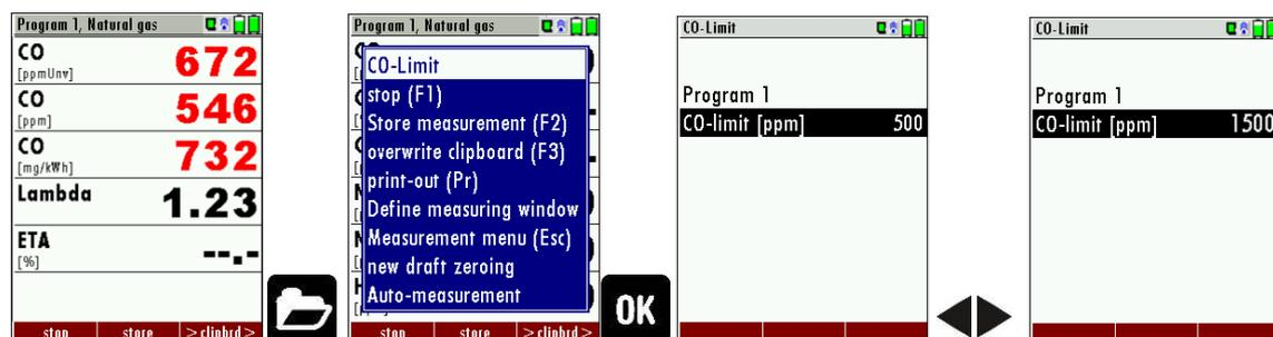
If the CO limit value is exceeded, the colour of the measured CO values changes (red).
