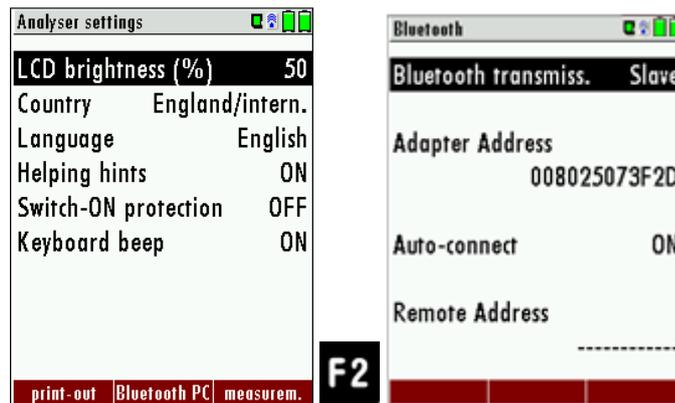
If RemoteData, OnlineView or MRUConnect (PDA) with Bluetooth is used, the SLAVE mode must be selected. The auto connect mode must be switched OUT.
