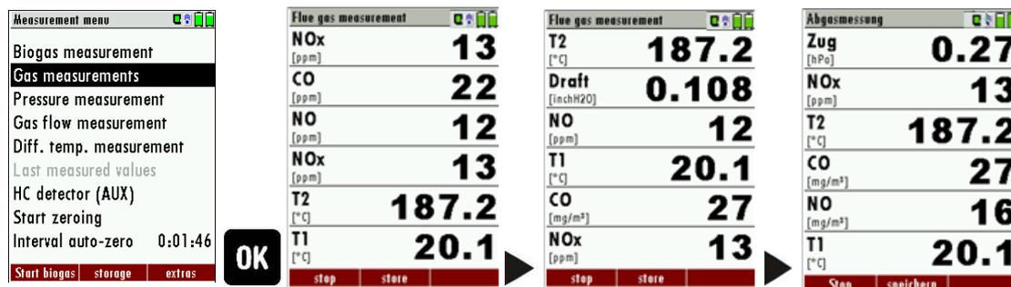
There are direct measured values available such as Oxygen and Temperature as well as calculated values such as dew point, efficiency and CO<sub>2</sub>. You will also find the same measurement value in different calculated values such as CO in ppm or CO in mg/kWh.
