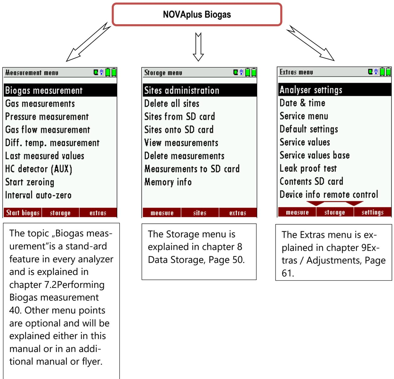
You can jump in between the 3 main menus with the 3 function keys (according to the displayed name on the screen).
