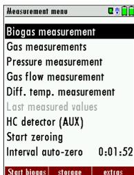
You can start a measurement with the previously set measurement parameters directly from the Measurement menu.
